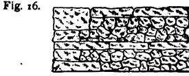
Fig. 16. Laced Coursed. —Horizontal bands of stone or bricks, interposed to give stability.
